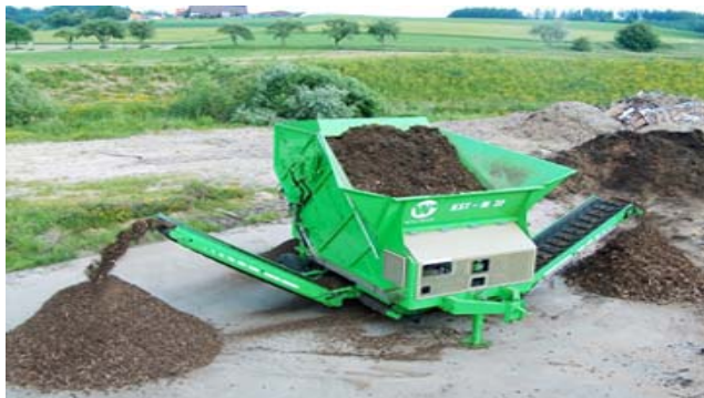
Fig. 4.1. Compost sorting plant
