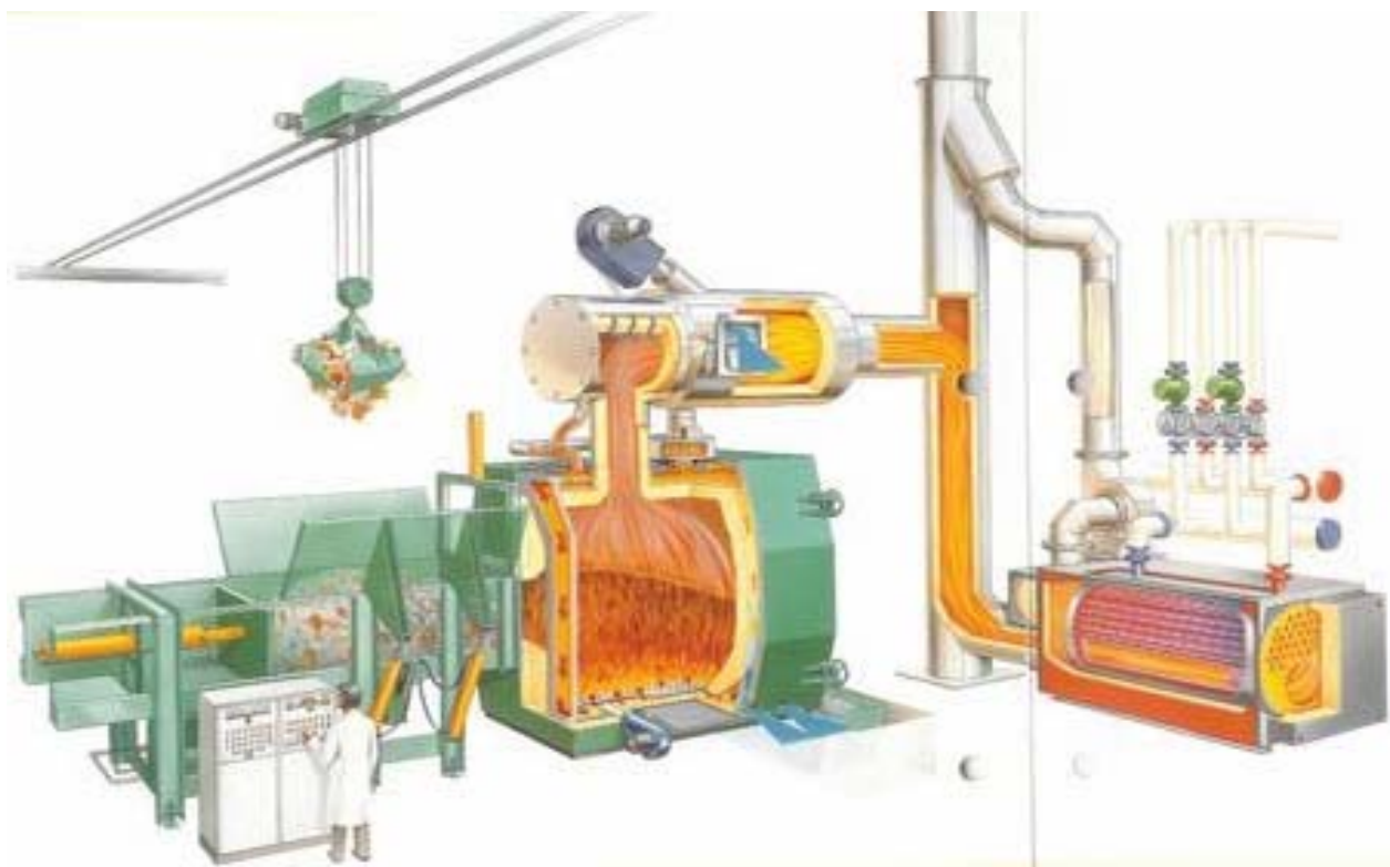
Fig. 3.1. Waste incineration installation type HOVAL MULTIZON
